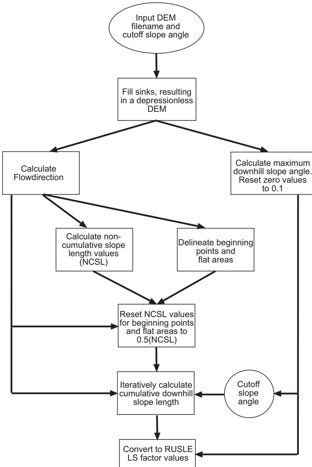
**Figure 1.** Flowchart illustrating the process of calculating cumulative downhill slope length (and LS values) for use in the RUSLE.
