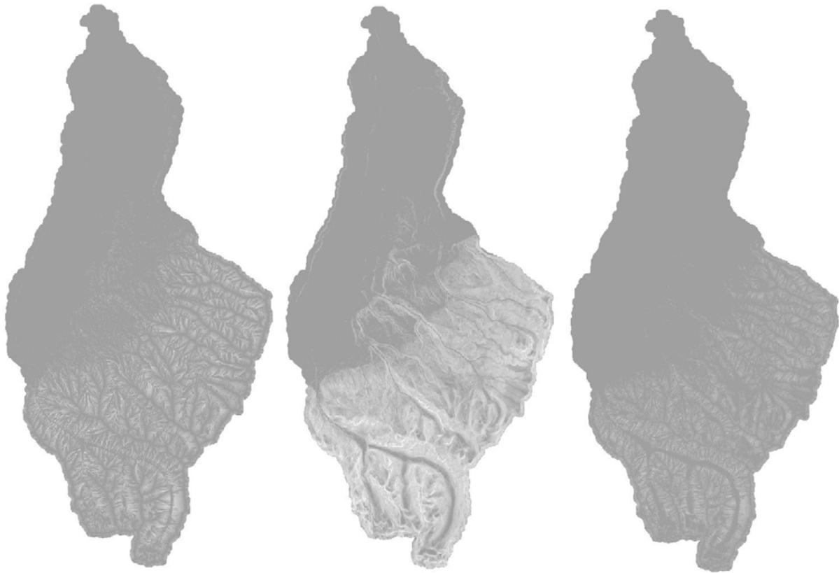
**Figure 2.** *Grids of the L constituent, S constituent, and LS factor, respectively, for the Lamoille Creek watershed in northeastern Nevada, USA.*
